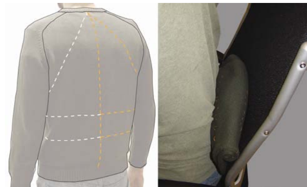
Figure 4. One student with a chronic sports injury created a garment for body awareness - a sweater, stitched with a pattern offering directions for folding into a back support device. Embedded vibrating motors occasionally remind the user to move and reorient his posture (by John T. Pugh).
